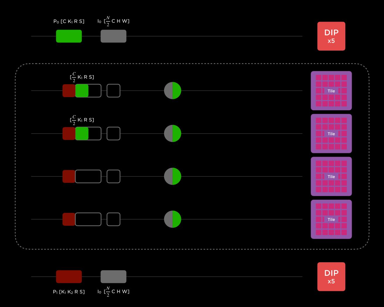
Discard Replicated Parameters and Input for Minimal SRAM Footprint
