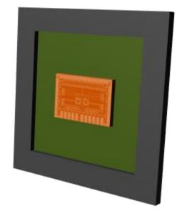
> 16Tbps cell-based fabric switch ASIC
