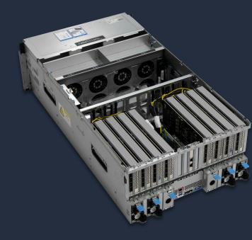
Integrating eight boards into a standard 4U rack form-factor, the proposed server-level solution extends the capability of the LightTraders up to - 128 TFLOPS / 512 TOPS
