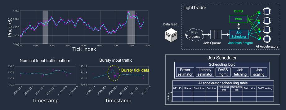
The advanced scheduling features retain high throughput for tick-by-tick inference jobs even for the bursting input query
