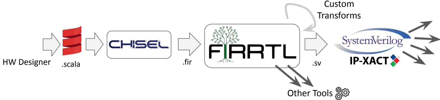
Building **robust** tools is **fast and cheap** using the FIRRTL IR:
